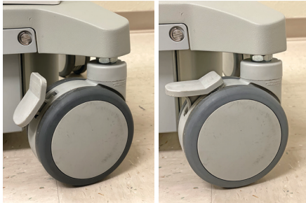
Figure 4: Caster Locked (left) and Unlocked (right)
