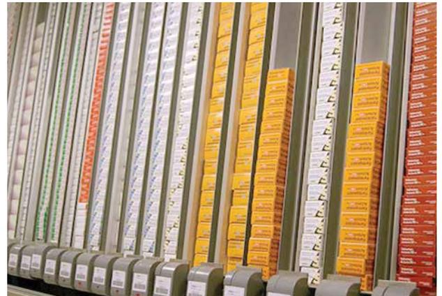
*In the highest volume systems space-saving storage is essential. RoboPharma's unique FastMover Channels are vertical to take advantage of deep stacking.*
