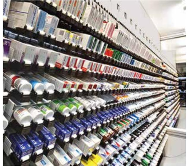
*Replenishment is logical, fast, and uncomplicated. Technicians scan the medication's bar code, enter the quantity to load, and insert medication packets. RoboPharma software guides the replenishment and tracks inventory levels.*
